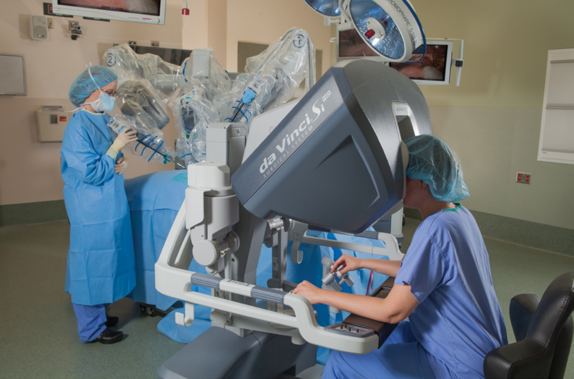
A robotic myomectomy being performed. The surgeon sits at the console while an assistant holds an instrument at the operating table. (©2018 Intuitive Surgical, Inc.)
